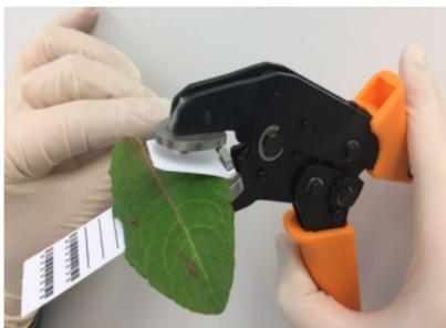
Remove a PhytoCard from its sterile pack and lift the flap covering the absorbant card. Slide the card fold-first into the groove of the jaws.
