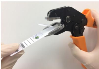
The jaws of the crusher tool can lock for easy packing. To unlock them, squeeze the handles fully and release. The jaws will then open.
