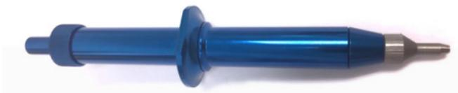
Samples are taken using a standard Harris punch with a 3 mm hole cutter. To take a sample with the punch tool, gently press down onto the card with the metal cutting tip until the punch is taken. A twisting motion will help.
